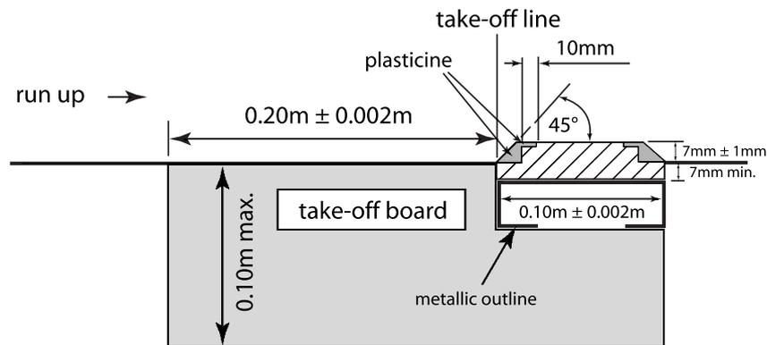
**Figure 184a- Take-off board and plasticine indicator board**
