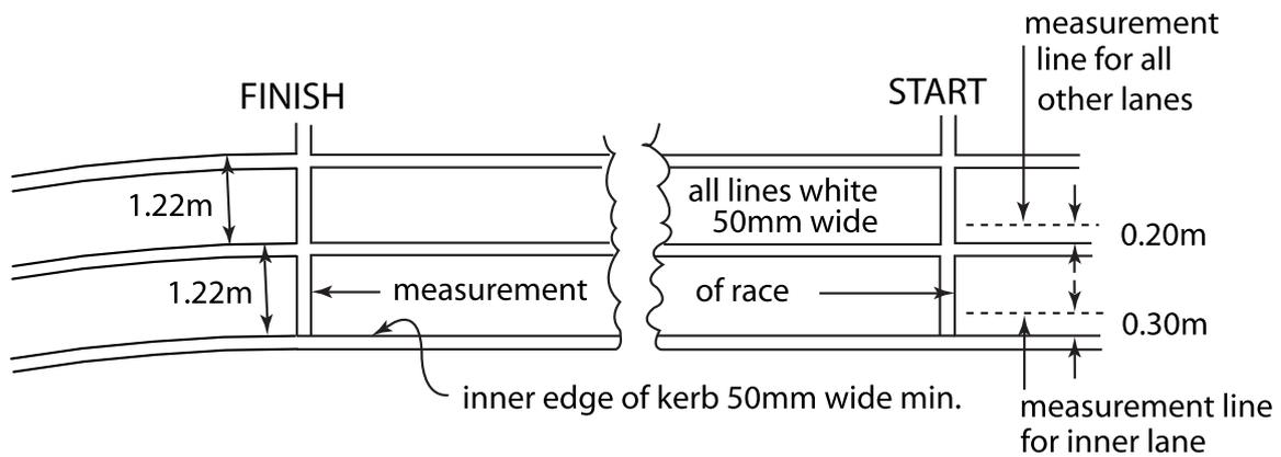
**Figure 160- Track measurements (infield view)**
