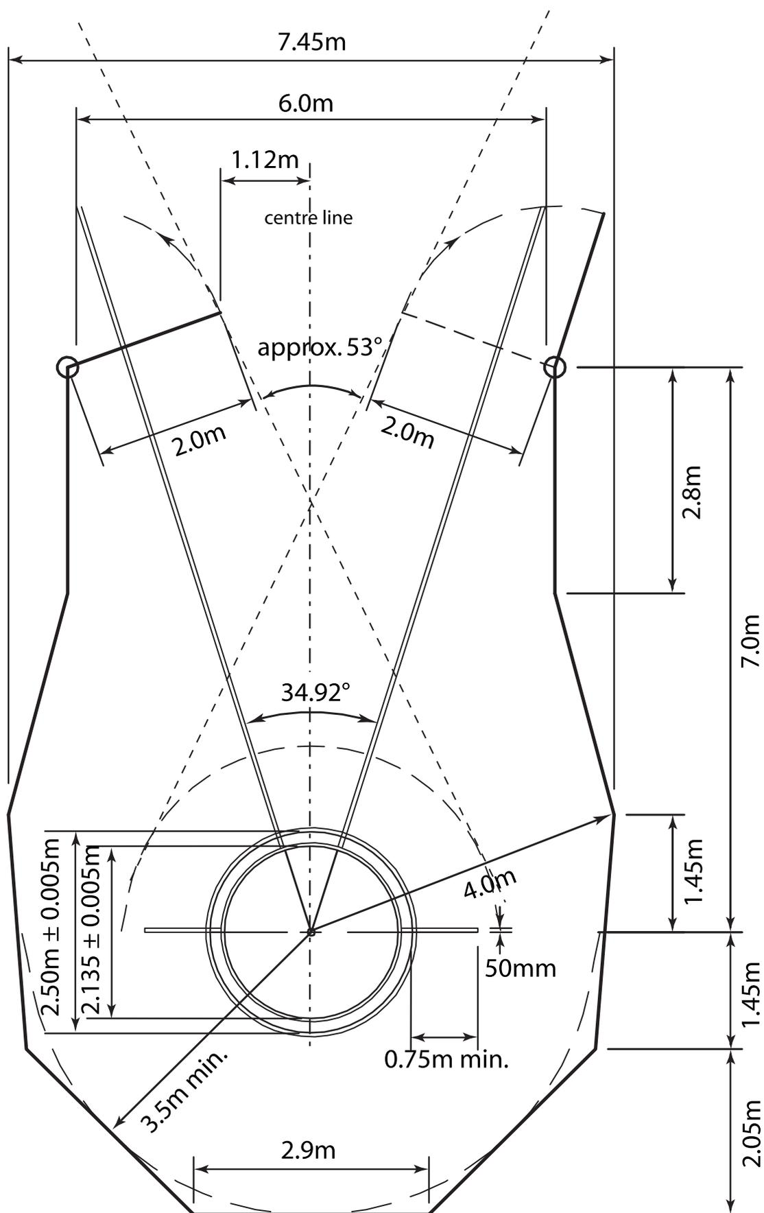
**Figure 192a - Cage for Hammer and Discus Throw with concentric circles**
